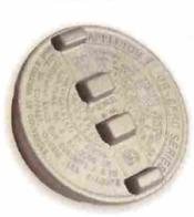
The Hardy Vibration Switch provides high- end vibration protection in a low profile, Class 1 Division 1 package. The vibration switch, which is mounted directly to rotating or reciprocating equipment, monitors equipment vibration and activates an onboard relay when a high level is reached. The Hardy Vibration Switch uses a piezoelectric crystal and state-of-the-art electronics to provide the highest degree of precision in this stand-alone monitoring system.
